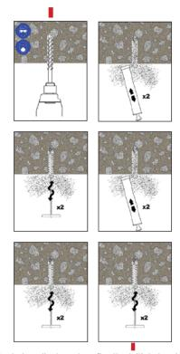
If the hole collects water after the initial cleaning, this water must be removed before injecting the resin.
